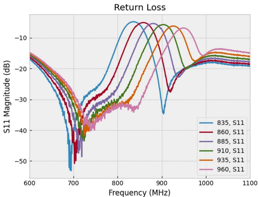
**Figure 3. Filter Return Loss vs Center Frequency**
