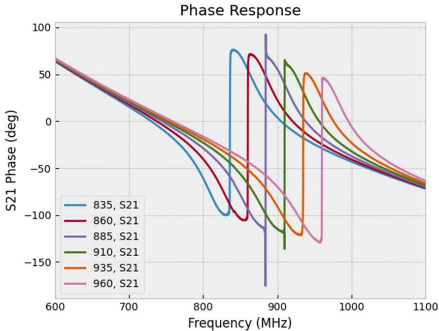
**Figure 4. Filter Phase vs Center Frequency**
