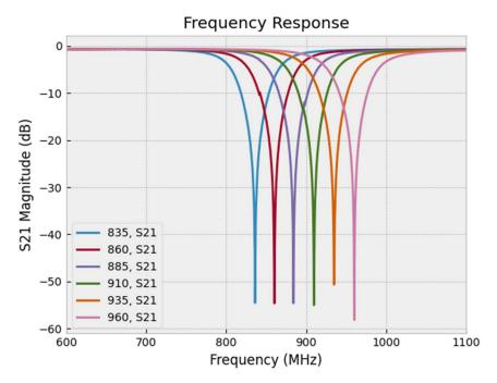
Figure 2. Filter Insertion Loss vs Center Frequency
