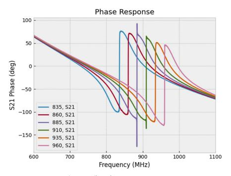
Figure 4. Filter Phase vs Center Frequency
