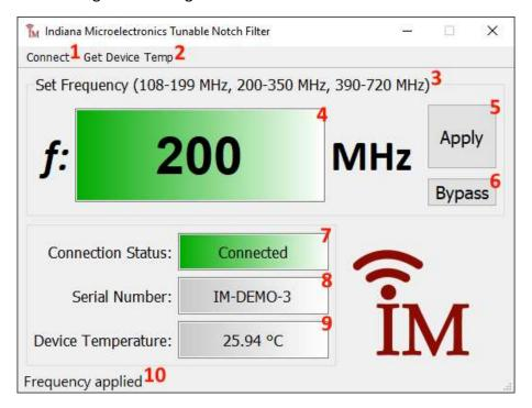
Figure 6. Tunable Notch Filter Control Software
