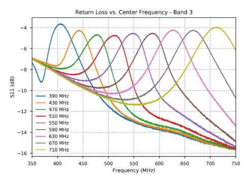
Figure 7. Filter Return Loss vs Center Frequency – Band 3
