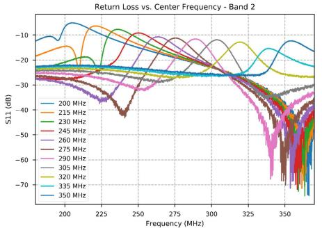
Figure 6. Filter Return Loss vs Center Frequency – Band 2
