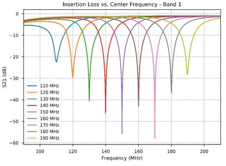
Figure 2. Filter Insertion Loss vs Center Frequency – Band 1
