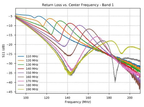
Figure 5. Filter Return Loss vs Center Frequency – Band 1
