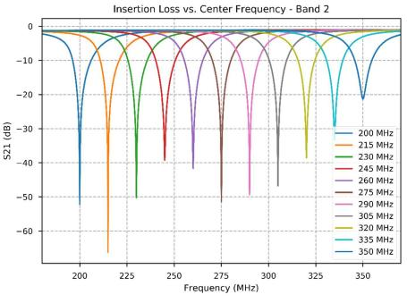
Figure 3. Filter Insertion Loss vs Center Frequency – Band 2
